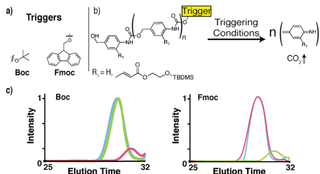
Figure 2. Triggered depolymerization of polymers. (a, b) Scheme depicting (a) the triggers and (b) the polymers and disassembly chemistry. (c) GPC traces showing disassembly of the polymers after removal of the triggers. Green: 10% piperidine, THF, 15 min. Red: 1:1 TFA/CH 2 Cl 2 , 15 min. Blue: unexposed polymer.
